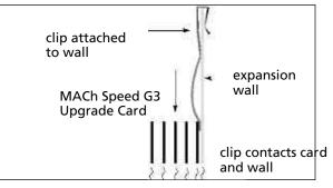
Cutaway view of the installed grounding clip
